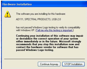
3. Hardware Installation Click 'Continue Anyway'
